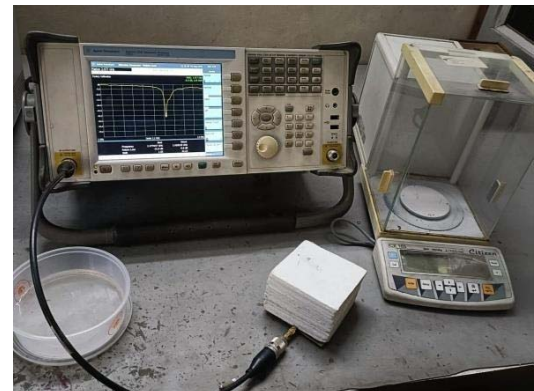
Figure.2 Paper arrangement on microstrip patch antenna. (a) Microstrip patch antenna structure. (b) Patch antenna with Paper sample placed.(c) Patch antenna with paper sample and pressure block. (d) Experimental Setup.
